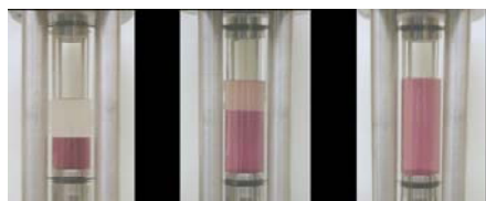
Figure 1. Biphasic system FC75-toluene 0b of CO 2 , in the middle 32b, and in the right monophasic
